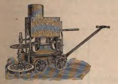
suitable electric power, can perform surfacing in a much more satisfactory manner and at an expense hardly to be compared with the old hand method. It is also serviceable for polishing large granite and marble surfaces.
